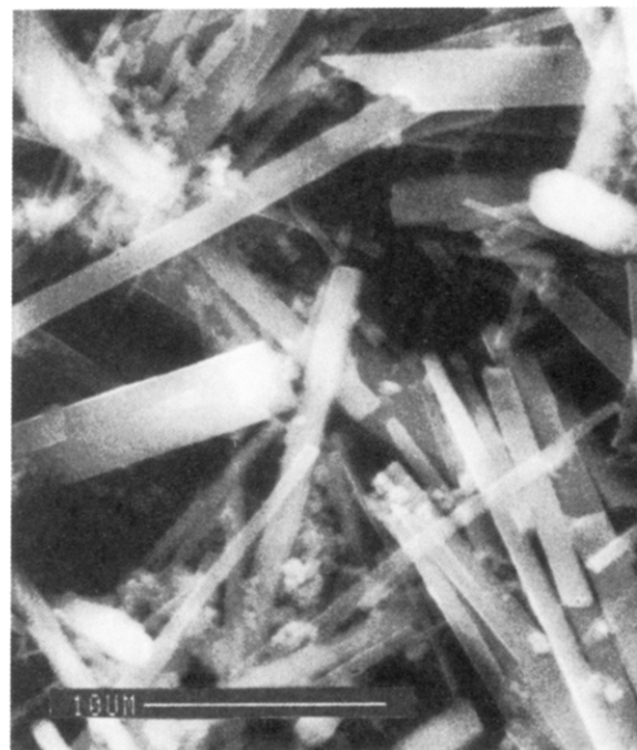
Figure 3. Scanning electron microscope photographs of titanium dioxide–sodium phosphate reaction products.
